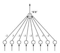
You can imagine that this network is one of the parts making up a demon. If the bottom row of toy neurons is connected to short-term memory, the top one detects whether short-term memory contains an instance of the symbol B. And on page 102 is a network for a demon-part that *writes* the symbol B into memory.
