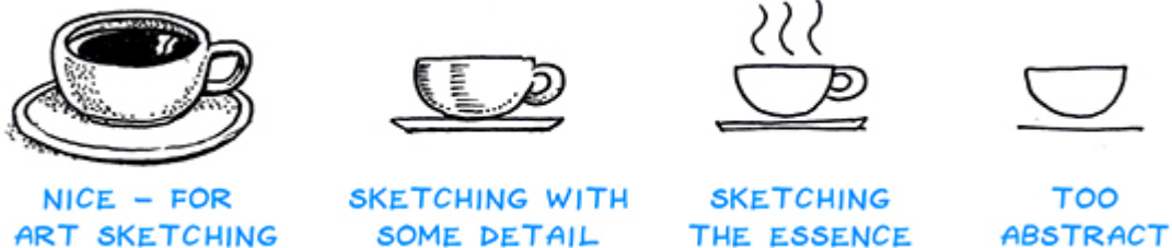
Figure 5-17. Sketching at different levels of fidelity: From higher fidelity (more photorealistic) on the left, to low fidelity on the right. We'd be here all day if we always sketched things like the coffee cup on the left, but if the sketch is too simple (far right), we miss some important details and a little bit of character. Aim for the fidelity level of the second cup from the right.
